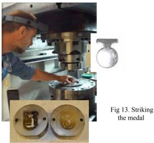
imprint the desired design on the coin's surface. This cold flow metal processing produces a sharper, more distinct image than is possible with the more commonly used metal casting process (Fig 13).
