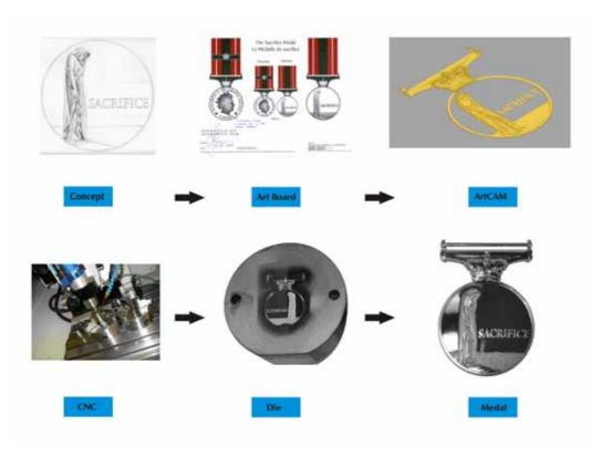
Fig 2. How it is made
