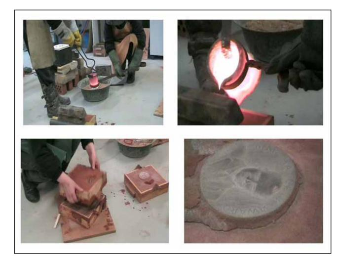
Fig 4. Sand casting demonstration
